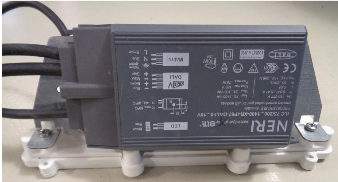
Photograph No. 3 Luminaire overview (side view, LED Driver's details)
