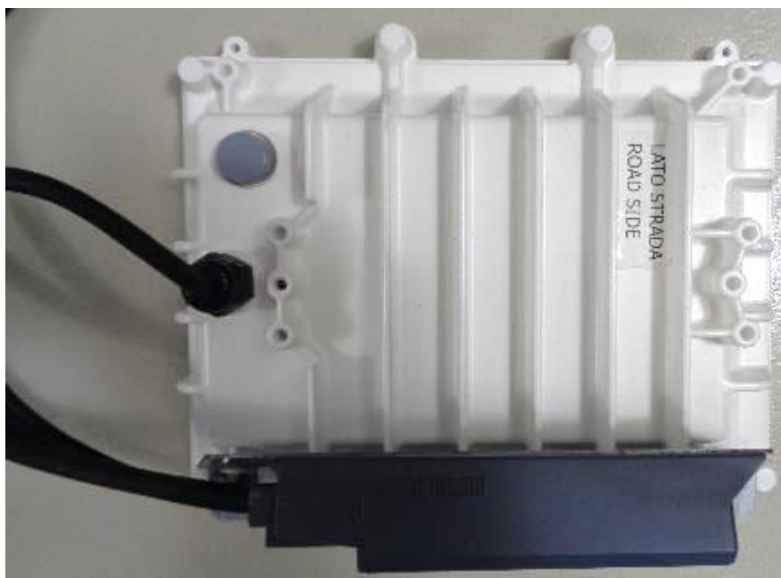
Photograph No. 2 Luminaire overview (back side, LED module and Driver)
