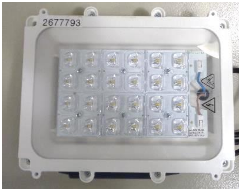
Photograph No. 1 Luminaire overview (front side, LED module)
