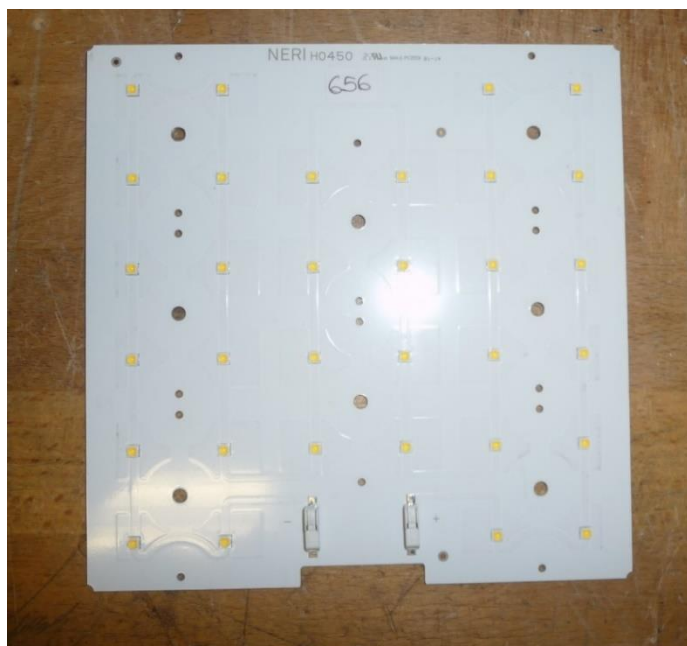
Photograph No. 6 View of the integral LED module (32 LEDs)
