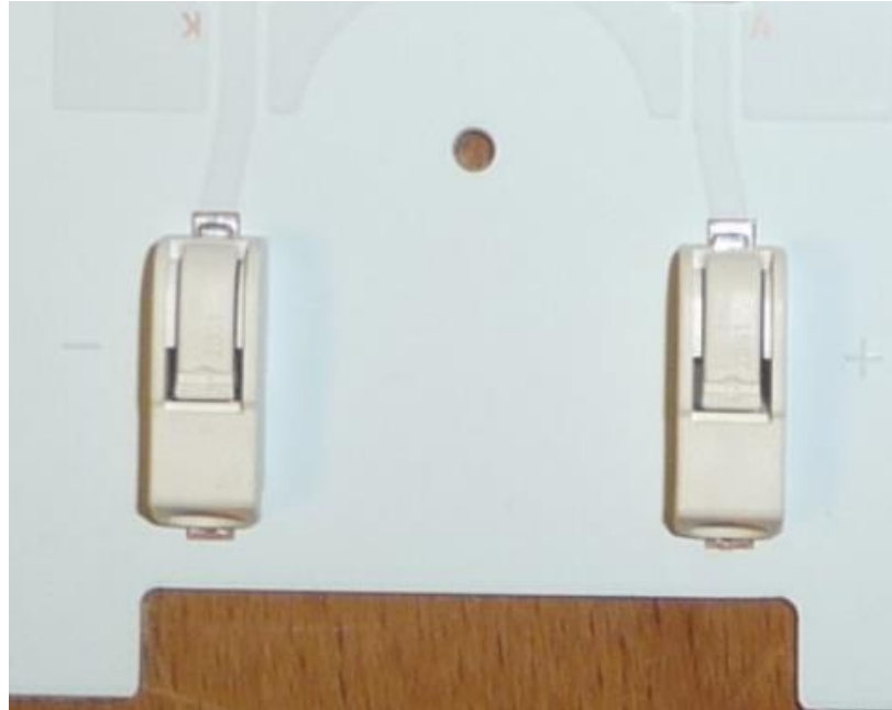
Photograph No. 9 LED module supply terminals
