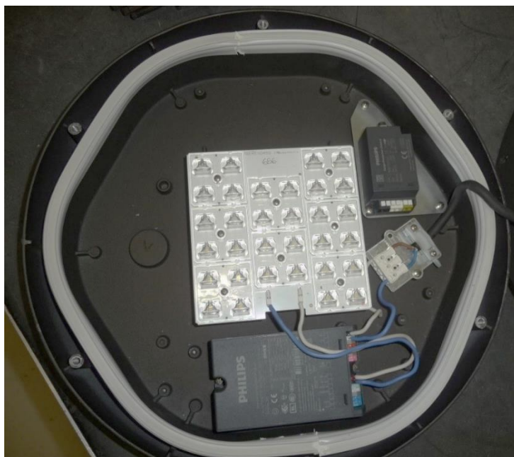
Photograph No. 5 View of internal wiring
