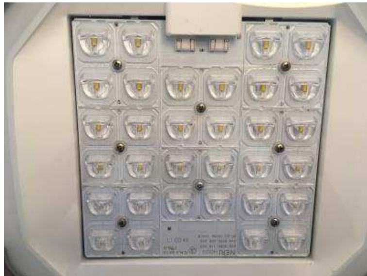
Photograph No. 4 – View of LED Chip and Lens.
